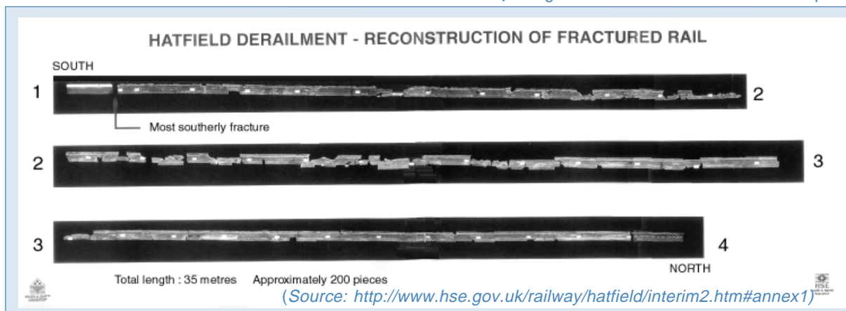
▼ Figure 3 - Rail broken into over 200 pieces
