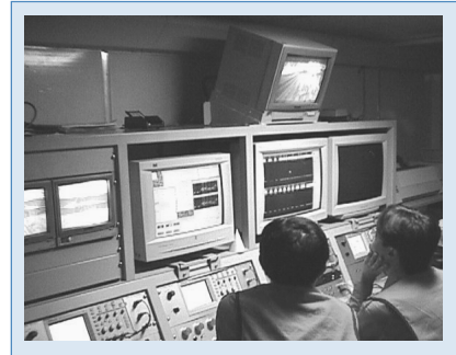
Figure 8 - Interior of ultrasonic testing vehicle
